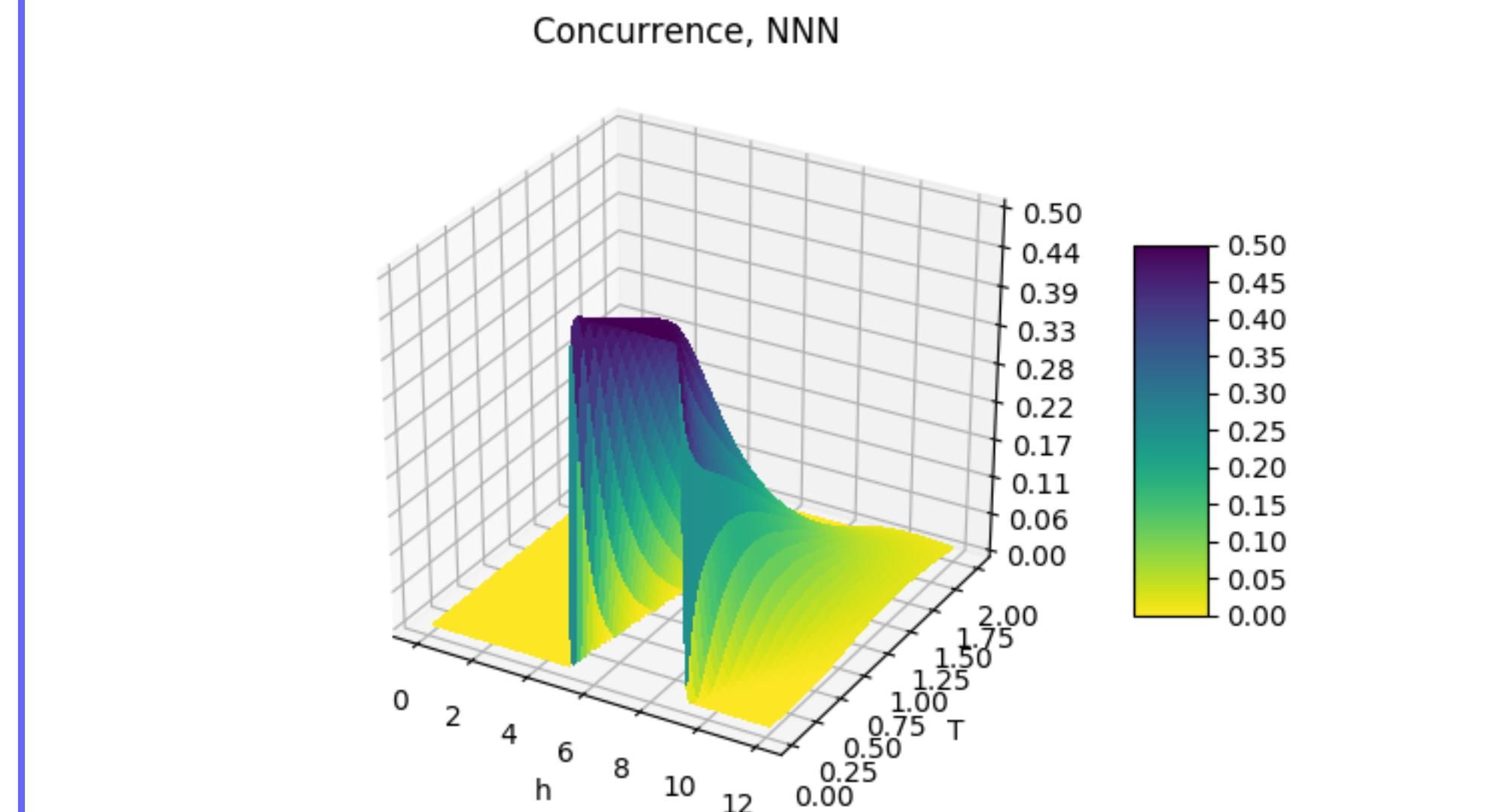
Density plots of the concurrence  $C_{nnn}$  as a function of magnetic field and temperature.
