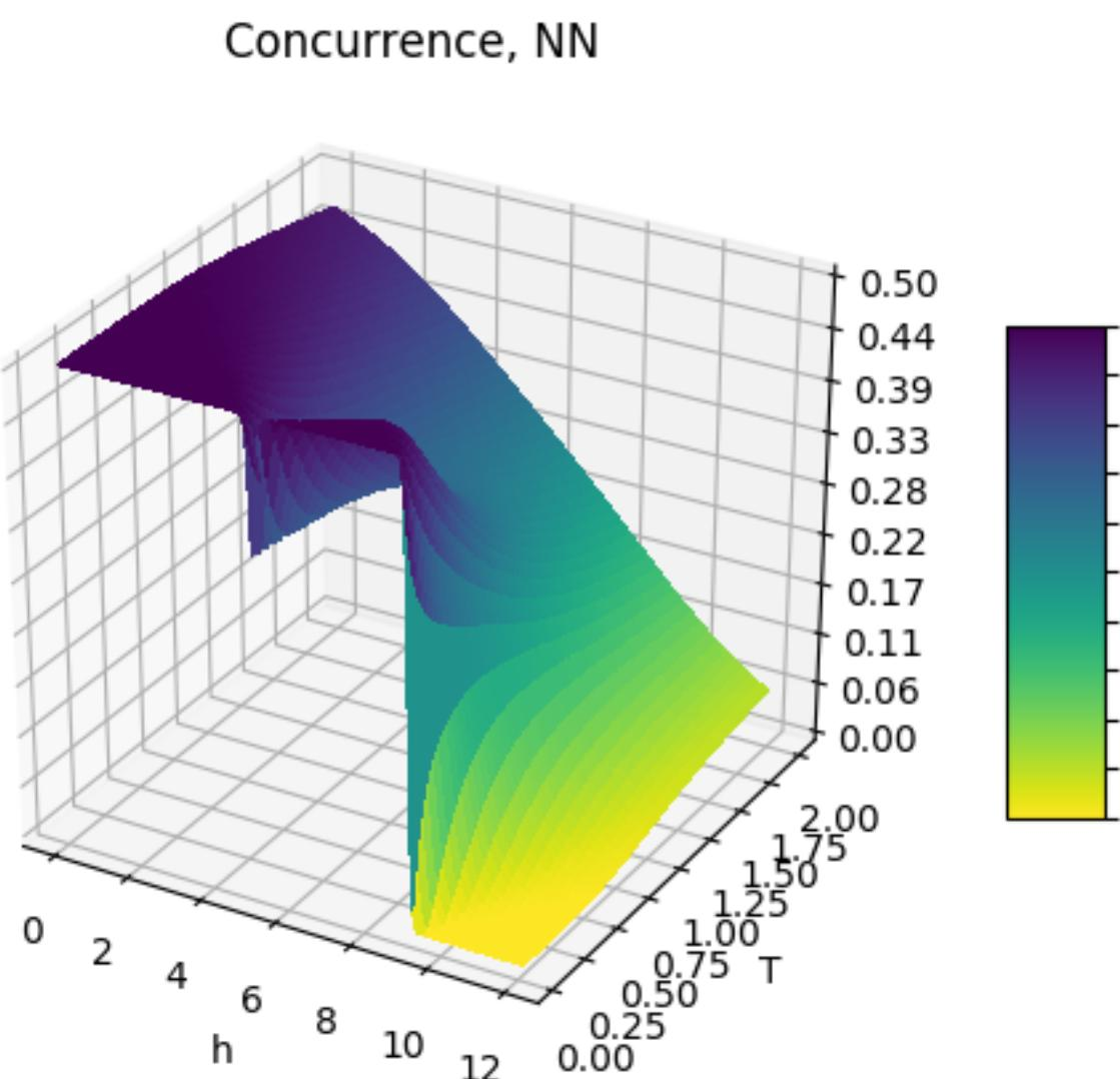
Density plots of the concurrence  $C_{nn}$  as a function of magnetic field and temperature.
